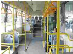
11. This is a shot of the front doorway showing how low the floor is on this bus. No step needed to enter the bus. This is the only place in Thailand that these low floor buses operate. Note this bus is branded as Shen Long inside but Golden Dragon on the outside.
